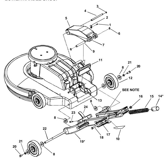
NOTE: GREASE ITEMS 14 AND SLIDE AREA OF 19 AS NECESSARY WHEN SERVICING.
