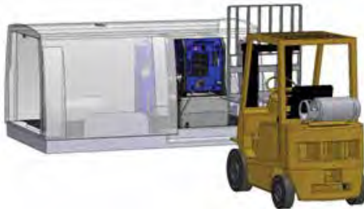
Figure 2-3. Use Forklift to Position Machine
