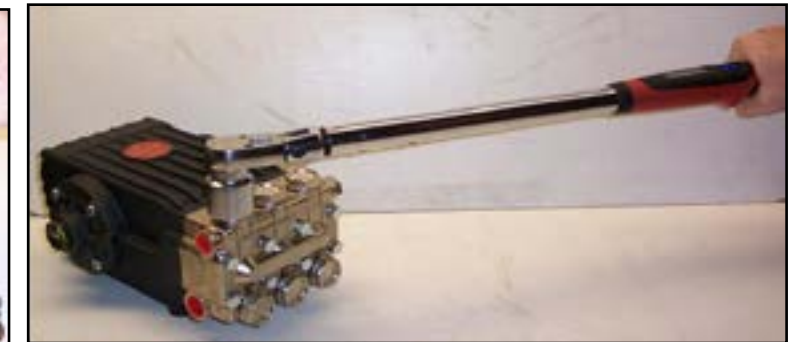
Figure 5-5. Replace Valve Cap and Torque to 95 ft lbs
