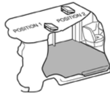
Figure 2-1. Location of Roof Vents in Vehicle
