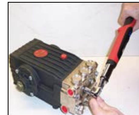
Figure 5-18. Torque Bolts to 22 ft. lbs
