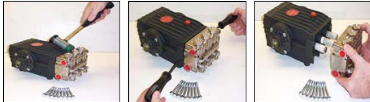
Figure 5-6. Separate Manifold from Crankcase
