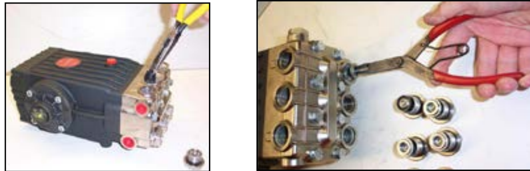
Figure 5-1. Remove Valve Cap and Valve Assembly
