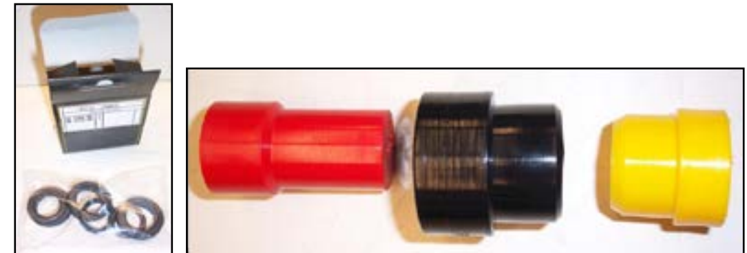
Figure 5-12. Seal Kit and Insertion Tool for Seal Installation
