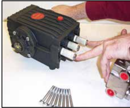
Figure 5-16. Re-install Manifold and Torque Fasteners
