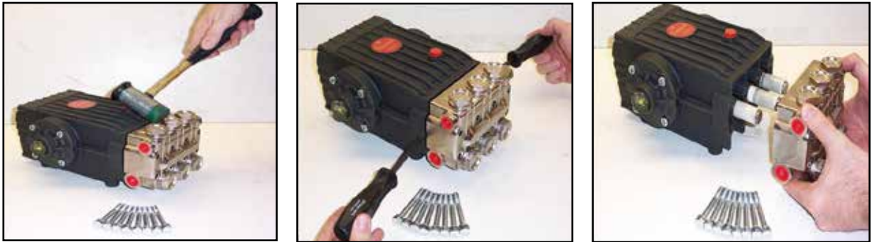
Figure 5-6. Separate Manifold from Crankcase
