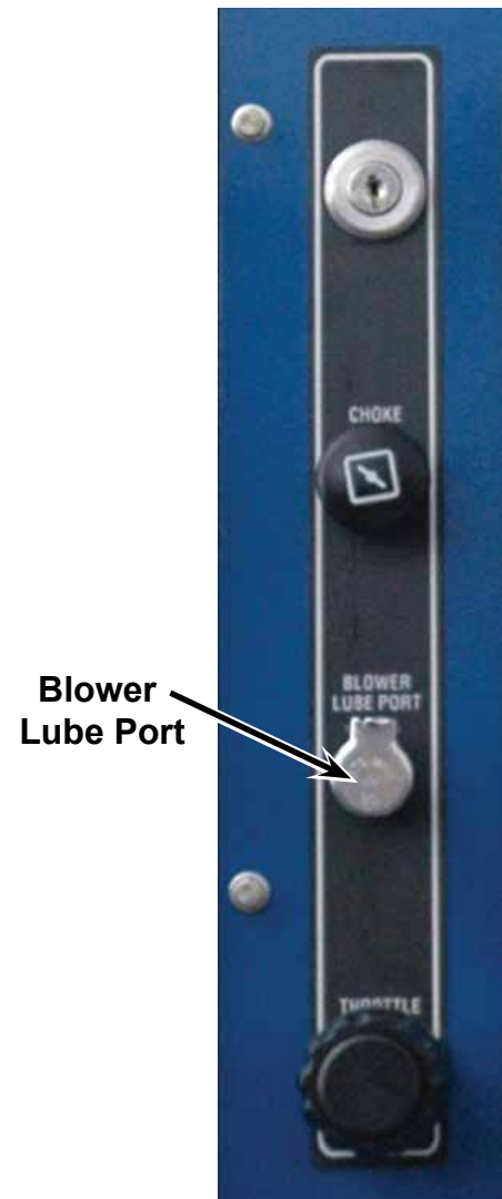
Figure 4-6. Location of Blower Lube Port
