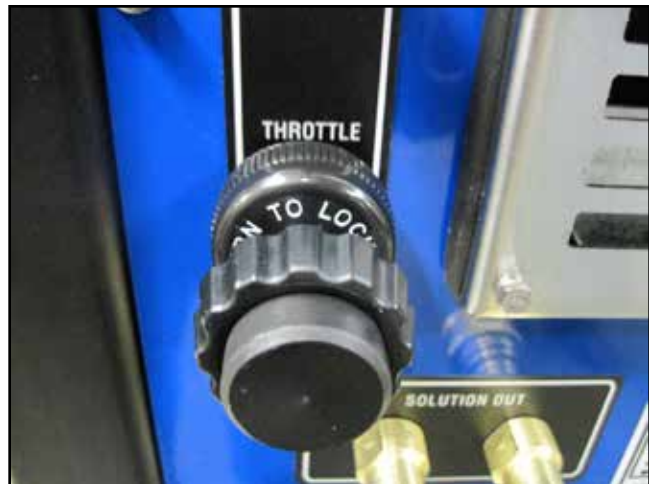
Figure 4-4. Turn Throttle Cable Knob Counterclockwise to Increase
