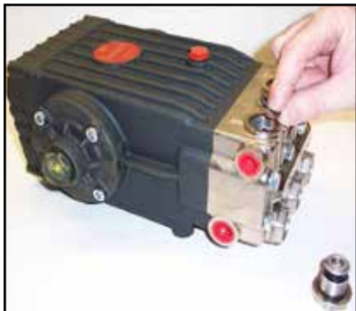
Figure 5-4. Apply Grease and Install Valves
