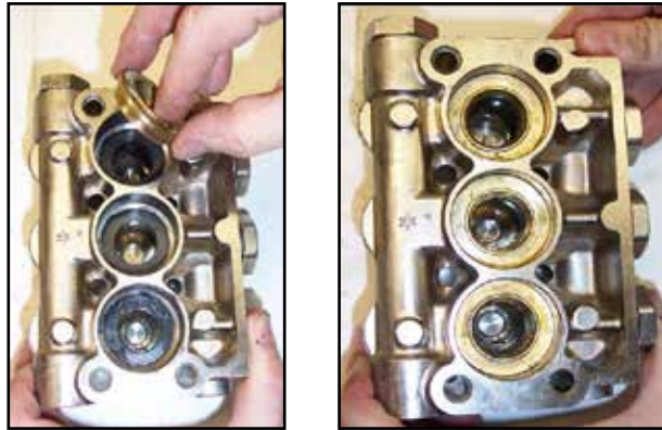
Figure 5-14. Install Retainers into Cavities
