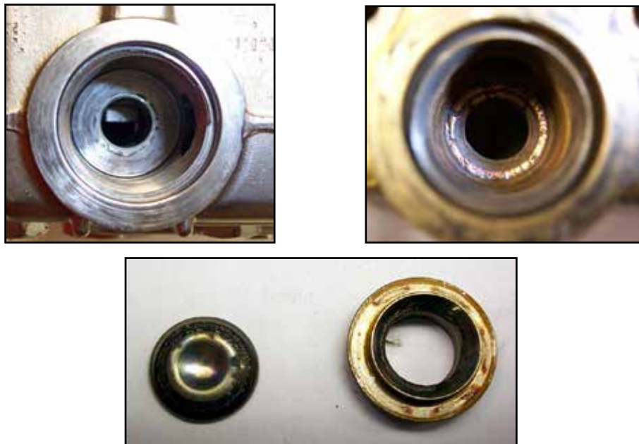
Figure 5-2. Inspect Manifold and Old Valves
