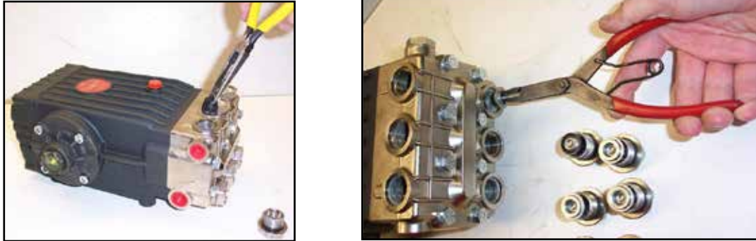
Figure 5-1. Remove Valve Cap and Valve Assembly
