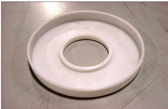
Figure 7 – Improved Bearing Shield, P/N 56380192
