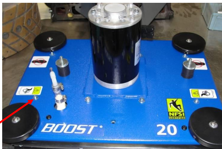
Figure 16 – Attaching Nuts to Lower Isolator Studs
