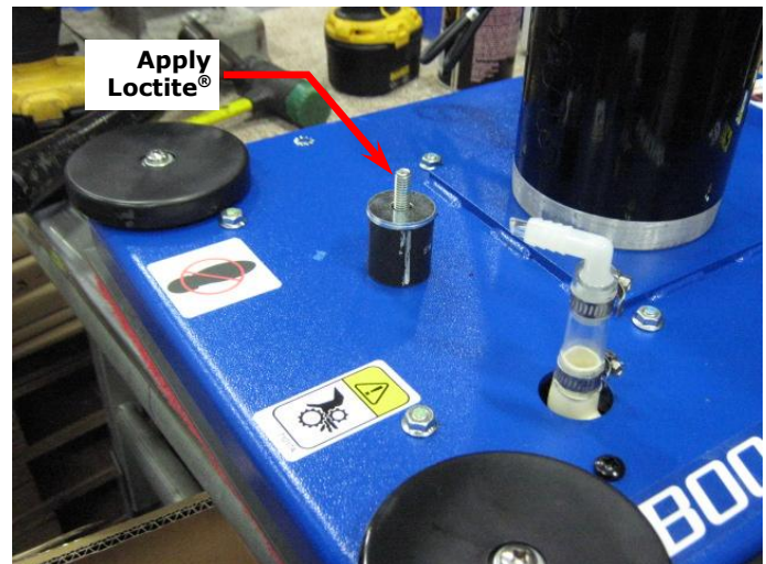
Figure 18 – Applying Loctite® to Upper Isolator Threads
