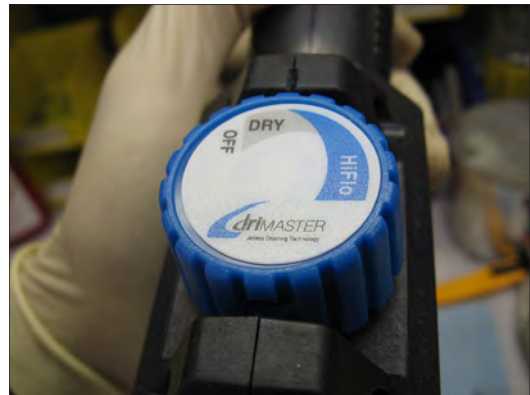
Figure 2-4. Turning Knob to “HiFlo” Position Forms Sheet of Water Across Bar Jet
