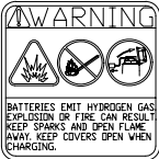
BATTERY CAUTION 86252520 PRV NO. 80885
