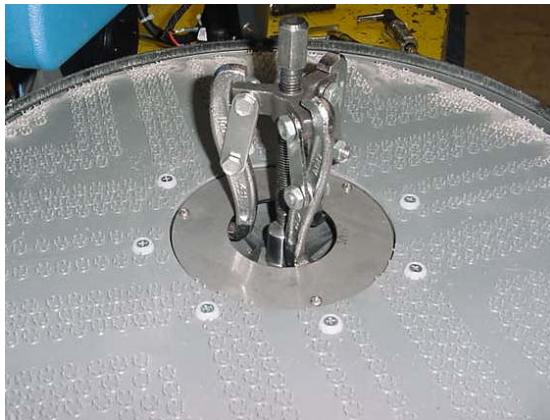
Use Gear puller to remove pad driver from motor shaft. Take care not to misplace motor shaft key.
