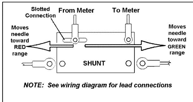
Check the amp range when nuisance tripping of the pad motor controller indicates that the shunt may be out of adjustment.
