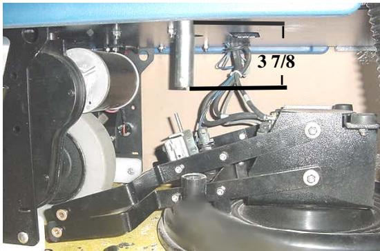
Reattach wires to motor and connect motor wire harness to frame harness. Tie wires in place. Set actuator barrel by rotating barrel up or down to set barrel at  $3\frac{7}{8}$  +0 -3/16 from top of frame to bottom of barrel.
