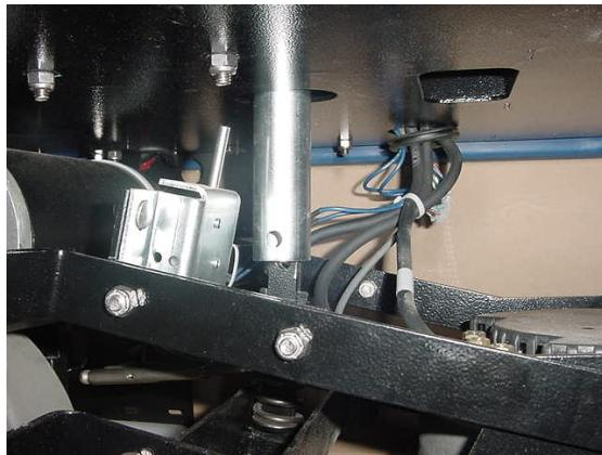
Reattach deck assembly to frame. Install actuator barrel on to spring retainer bars. Lift bottom of deck using your hand to align hole for clevis pin. Install clevis and rue ring. Turn machine on, raise deck, drive machine check that machine is working properly. If not recheck actuator barrel and reset again if needed.
