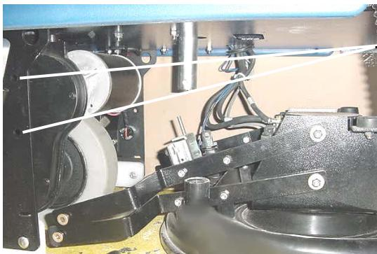
Remove the four bolts holding deck assembly onto frame. Two bolts on each side.
