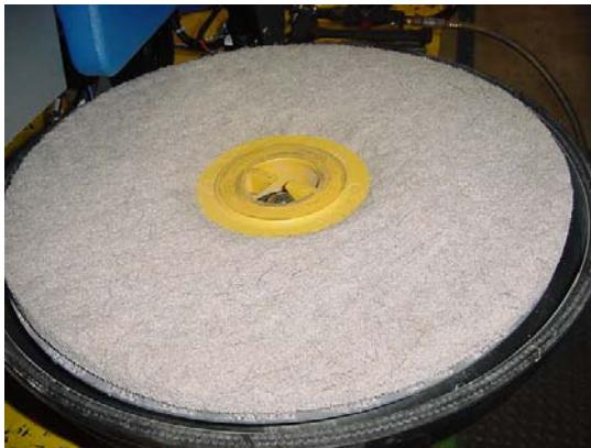
Slide deck out from under machine and turn deck assembly over on to motor. Remove pad lock and pad.
