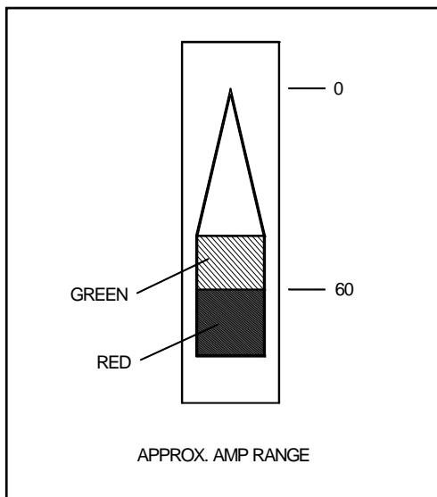
1. Connect a DC ampere meter to the positive battery lead. Running the machine with a pad, lower the pad to the floor until it is operating at  $60 \pm 5$  amps.
