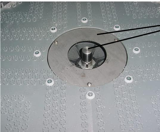
Attach metal ring (86082070 – PRV NO. 629000) using same screws that held pad lock keeper. Screw in spacer (862454470 – PRV NO. 739000) into motor shaft.
