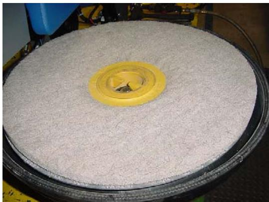
Install new pad driver, motor shaft key, spacer, washer and bolt. Then install pad lock keeper, pad and pad lock. Turn deck assembly over onto pad
