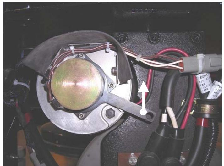
1. Mechanical over-ride disengaged
