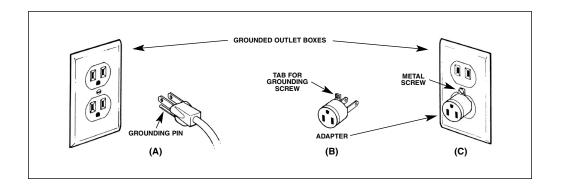
This machine must be grounded. If it should malfunction or break down, grounding provides a path of least resistance for electric current to reduce the risk of electric shock. This machine is equipped with a cord having an equipment-grounding conductor and grounding plug. The plug must be inserted into an appropriate outlet that is properly installed and grounded in accordance with all local codes and ordinances.
